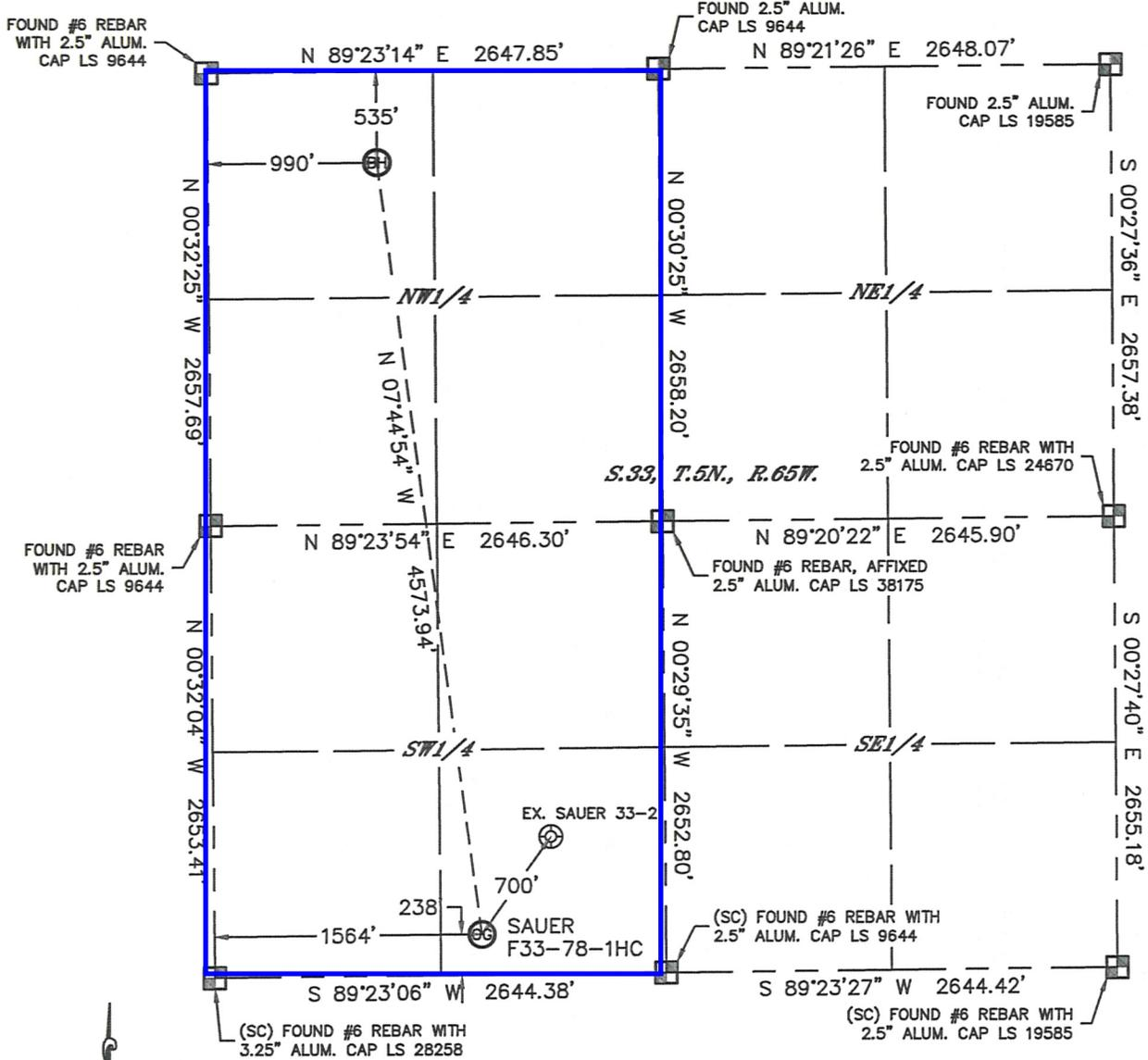
In accordance with a request from Jacob Rice with Noble Energy Inc., Lat40°, Inc. has determined the surface location of the SAUER F33-78-1HC to be 238' from the SOUTH line and 1564' from the WEST line and the bottom hole to be 535' from the NORTH line and 990' from the WEST line as measured at right angles from the section lines of Section 33, Township 5 North, Range 65 West of the Sixth Principal Meridian, County of Weld, State of Colorado.
