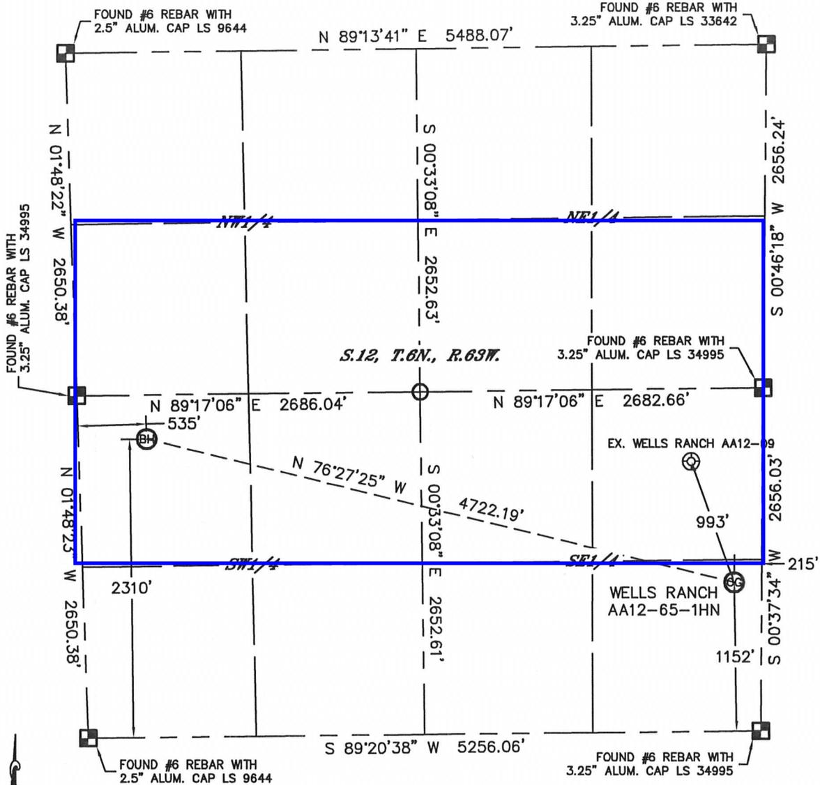
In accordance with a request from Sean Casper with Noble Energy Inc. Lat40°, Inc. has determined the surface location of the WELLS RANCH AA12-65-1HN to be 1152' from the SOUTH line and 215' from the EAST line and the bottom hole to be 2310' from the SOUTH line and 535' from the WEST line as measured at right angles from the section lines of Section 12, Township 6 North, Range 63 West of the Sixth Principal Meridian, County of Weld, State of Colorado.
