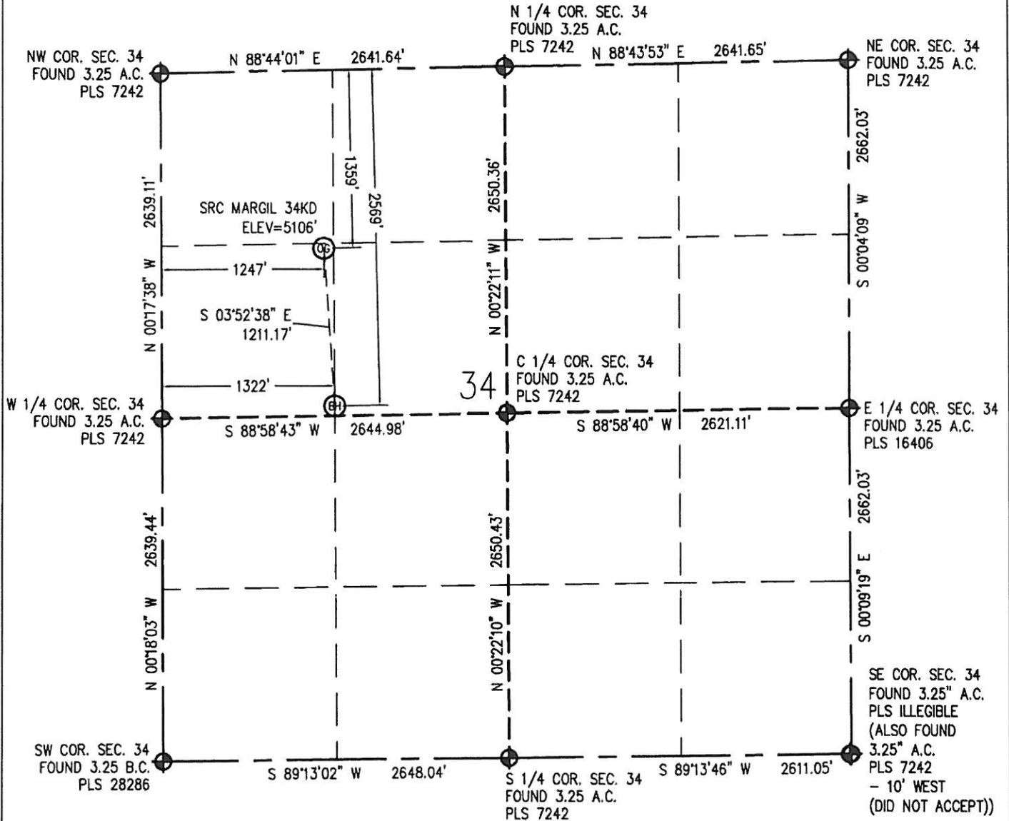
IN ACCORDANCE WITH A REQUEST FROM CRAIG RASMUSON - SYNERGY RESOURCES, BASELINE ENGINEERING CORP. HAS DETERMINED THE LOCATION OF THE SRC MARGIL 34KD TO BE 1,359' FNL AND 1,247' FWL, AS MEASURED AT NINETY (90) DEGREES FROM THE SECTION LINE OF SECTION 34, TOWNSHIP 4 NORTH, RANGE 68 WEST AND THE BOTTOM HOLE LOCATION TO BE 2,569' FNL AND 1,322' FWL OF SECTION 34, TOWNSHIP 4 NORTH, RANGE 68 WEST, 6TH PRINCIPAL MERIDIAN, WELD COUNTY, COLORADO.
