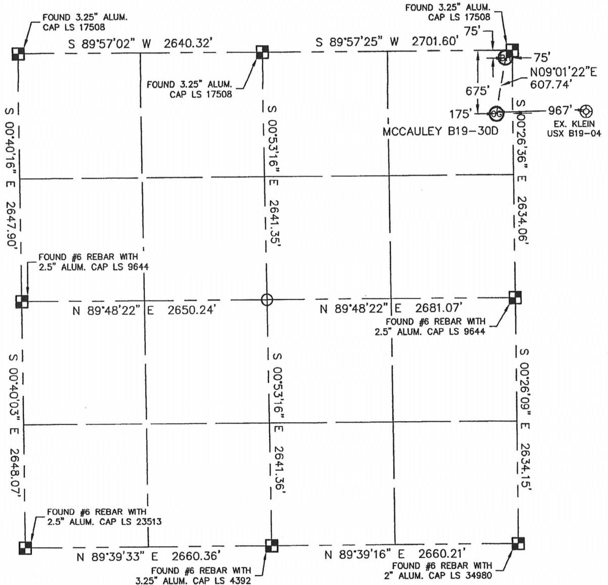
In accordance with a request from Matt Campbell with Noble Energy Inc., Lat40°, LLC has determined the surface location of the MCCAULEY B19-30D to be 675' from the NORTH line and 175' from the EAST line and the bottom hole to be 75' from the NORTH line and 75' from the EAST line as measured at right angles from the section line of Section 24, Township 5 North, Range 65 West of the Sixth Principal Meridian, County of Weld, State of Colorado.
