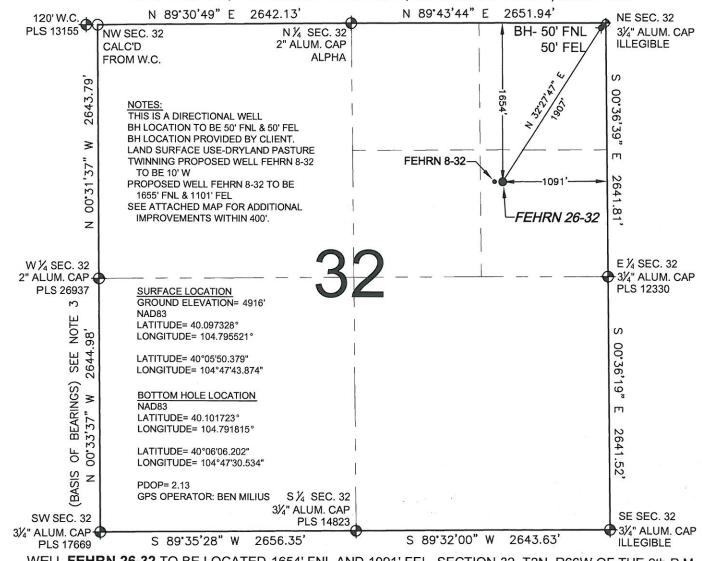
WELL FEHRN 26-32 TO BE LOCATED 1654' FNL AND 1091' FEL, SECTION 32, T2N, R66W OF THE 6th P.M.
