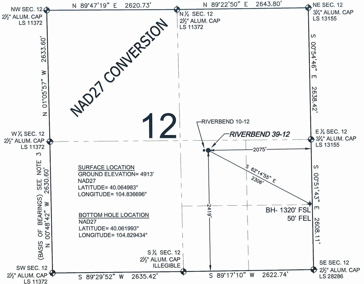
WELL RIVERBEND 39-12 TO BE LOCATED 2419' FSL AND 2075' FEL, SECTION 12, T1N, R67W OF THE 6TH P.M.
