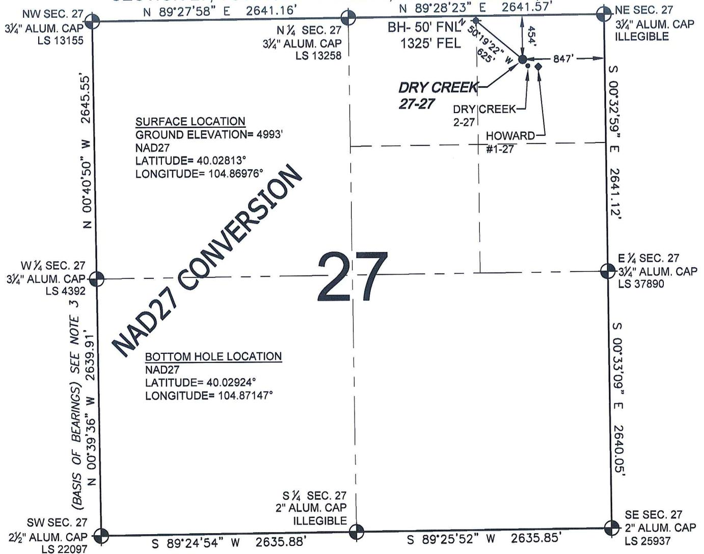
WELL DRY CREEK 27-27 TO BE LOCATED 454' FNL AND 847' FEL, SECTION 27, T1N, R67W OF THE 6th P.M.
