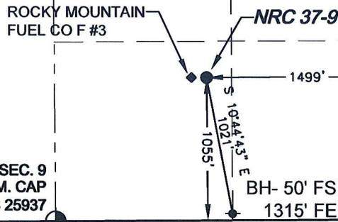
WELL NRC 37-9 TO BE LOCATED 1055' FSL AND 1499' FEL, SECTION 9, T1N, R67W OF THE 6TH P.M.
