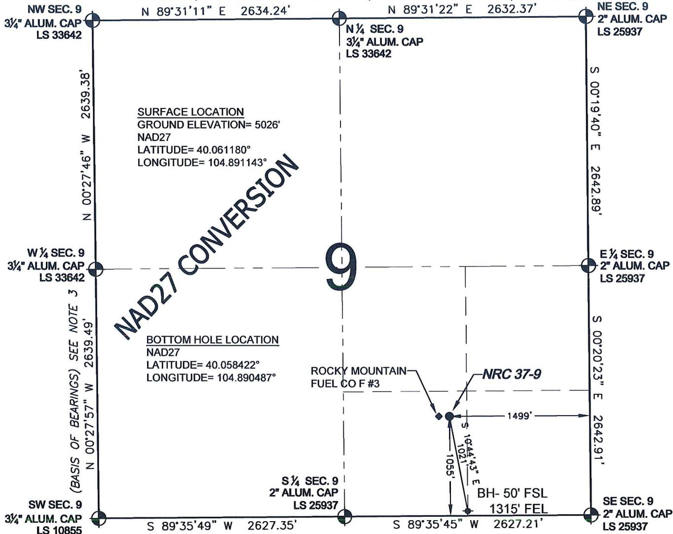
WELL NRC 37-9 TO BE LOCATED 1055' FSL AND 1499' FEL, SECTION 9, T1N, R67W OF THE 6th P.M.
