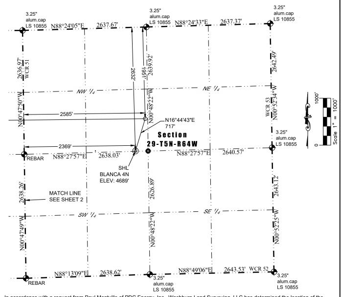
In accordance with a request from Paul Montville of PDC Energy, Inc., Washburn Land Surveying, LLC has determined the location of the BLANCA 4N well site to be SHL: 2632' FNL and 2369' FWL, (EP: 1951' FNL and 2585' FWL, BHL: 1951' FNL and 50' FWL), as measured at ninety (90) degrees from the section lines of Sections 29 and 30, Township 5 North, Range 64 West of the 6th Principal Meridian, Weld County Colorado.
