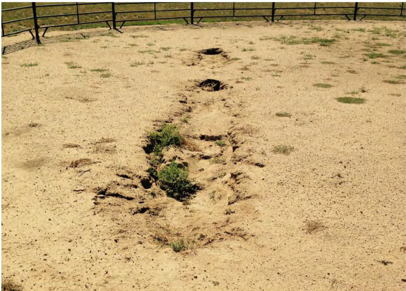
Figure 1 : Subsidence area in corral prior to excavation. View west.
