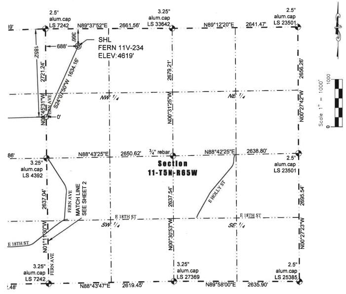
In accordance with a request from Paul Montville of PDC Energy, Inc., Washburn Land Surveying, LLC has determined the location of the FERN 11V-234 well site to be SHL: 366' FNL and 688' FWL, (EPL: 1852' FNL and 0' FEL), (BHL: 1852' FNL and 2530' FEL), as measured at ninety (90) degrees from the section lines of Sections 9, 10 and 11, Township 5 North, Range 65 West of the 6th Principal Meridian, Weld County Colorado.
