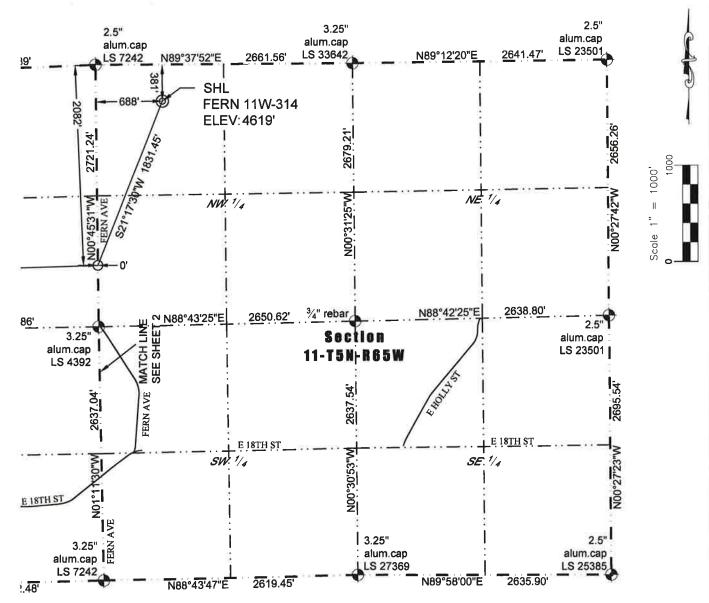
In accordance with a request from Paul Montville of PDC Energy, Inc., Washburn Land Surveying, LLC has determined the location of the FERN 11W-314 well site to be SHL: 381' FNL and 688' FWL, (EPL: 2082' FNL and 0' FEL), (BHL: 2082' FNL and 2530' FEL), as measured at ninety (90) degrees from the section lines of Sections 9, 10 and 11, Township 5 North, Range 65 West of the 6th Principal Meridian, Weld County Colorado.
