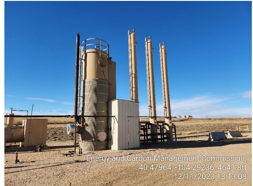
Photo 14 – Heater Treater and VRTs
