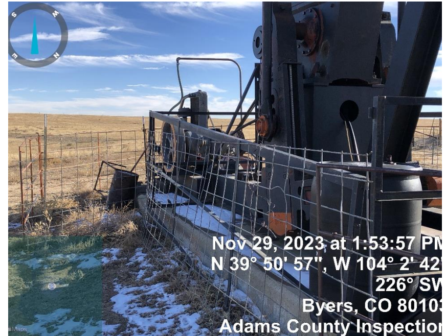
Photo#6 CA: No secondary containment for barrel
