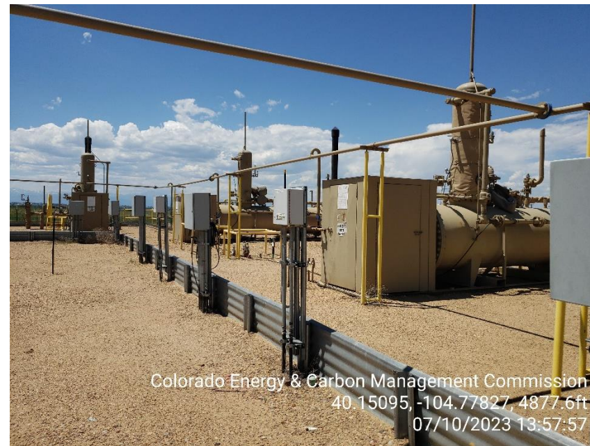
Photo 10 Horizontal Heated Separators.
