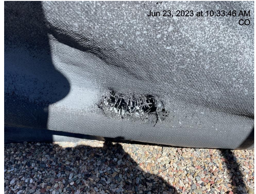
Photo # 1616 Hole in containment liner/liner needs maintenance
