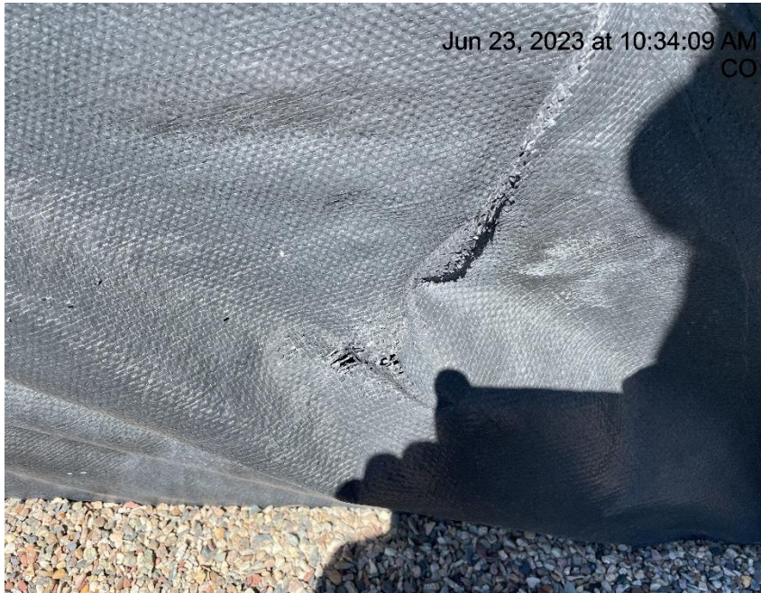
Photo # 1621 Hole in containment liner/liner needs maintenance
