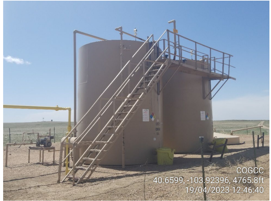
Photo 4 – Tank Battery
