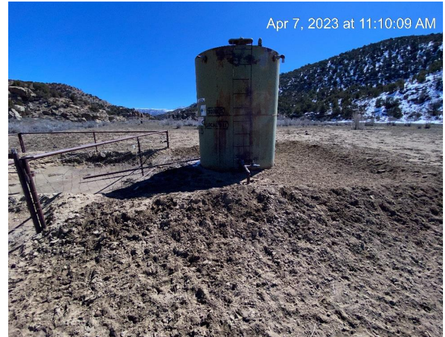
Produced water tank from pumping unit
