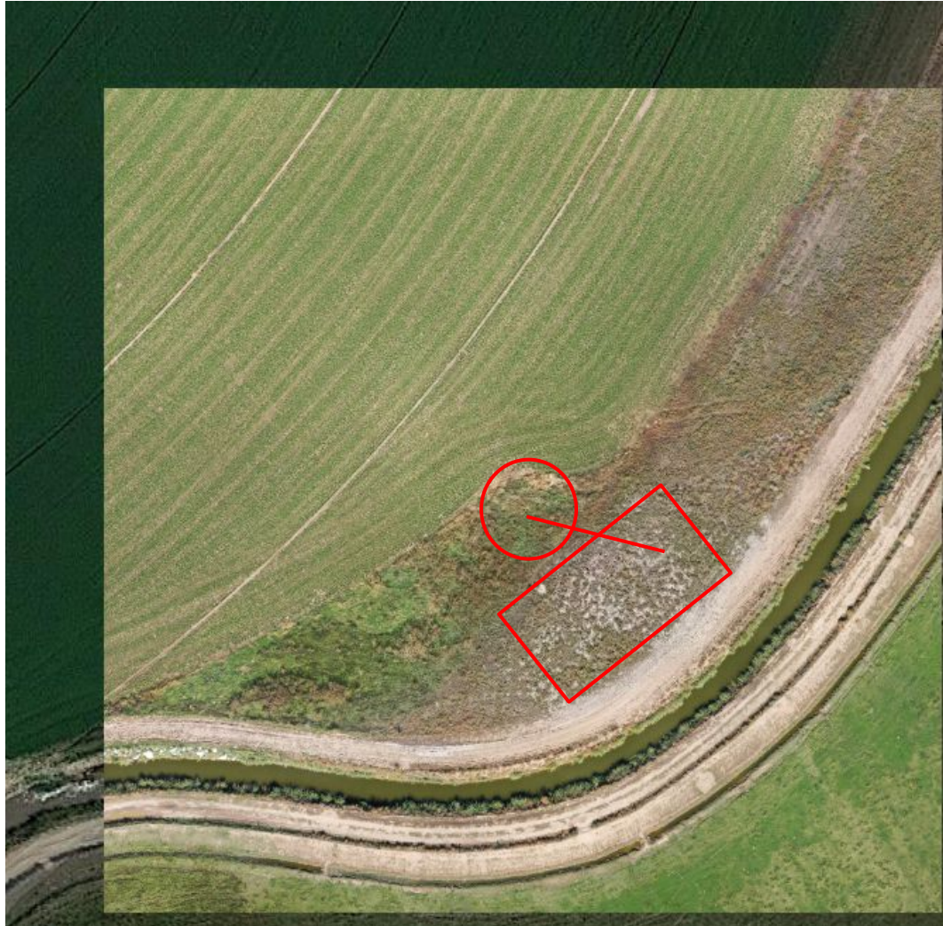
Photo 3. Orthomosaic drone aerial imagery taken from 200 ft (Oct. 2022). Illustrates growth on and around the well location (red circle), flowline (red line), and tank battery (red rectangle). Similar growth to range land near it.
