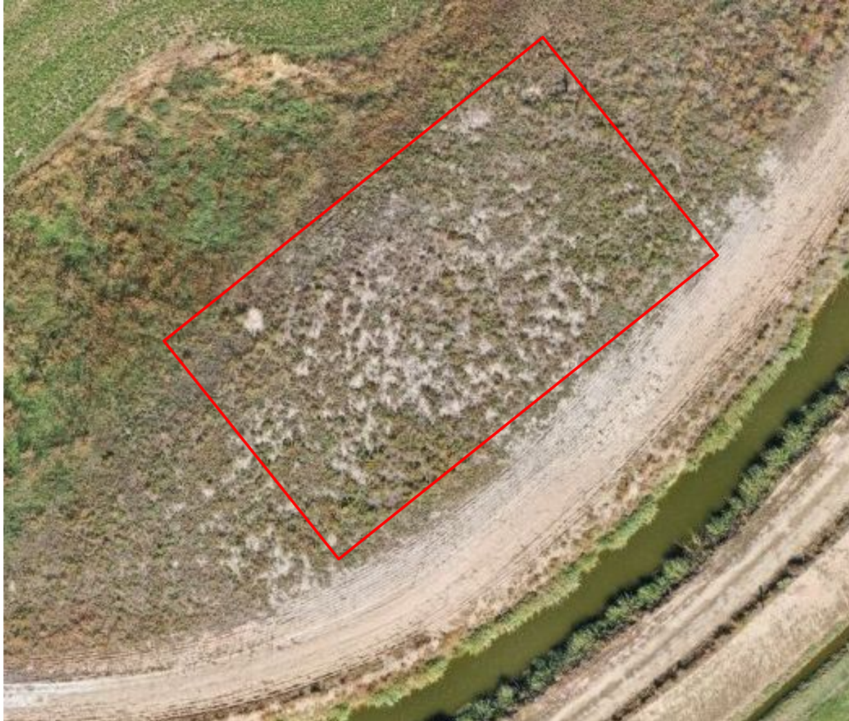
Photo 5. Zoomed in Orthomosaic taken from 200 ft (Oct. 2022). Illustrates less growth than surrounding range land on the tank battery (red rectangle).
