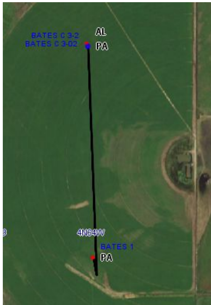
Photo 2. COGCC Online Map aerial imagery 2019 with subject well (blue dot), related wells (red dots), tank battery (south center) and flowlines (black lines).
