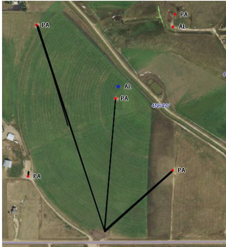
Photo 2. COGCC Online Map aerial imagery 2019 with subject well (blue dot), related wells (red dots), tank battery (south center) and flowlines (black lines).
