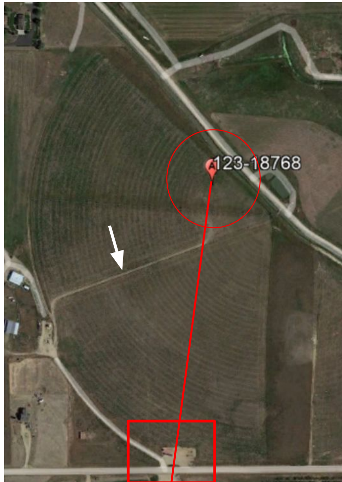
Photo 1. Google Earth aerial imagery taken 7/2019 during active operations. Photo illustrates the well location (red circle), tank battery (red rectangle), and access road (white arrow).
