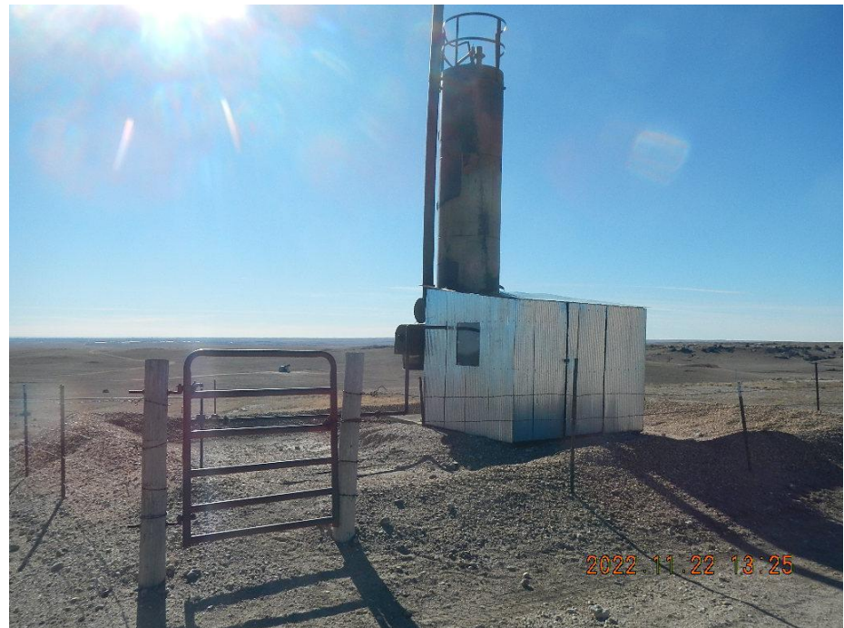
Photo 10. Vertical separator.
