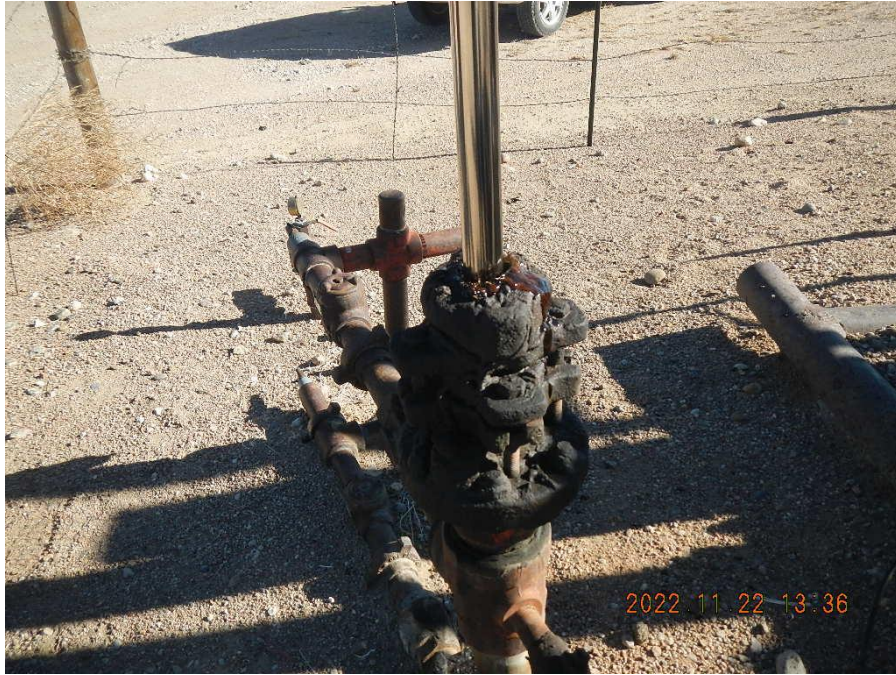
Photo 19. Paraffin and oil build up at stuffing box.
