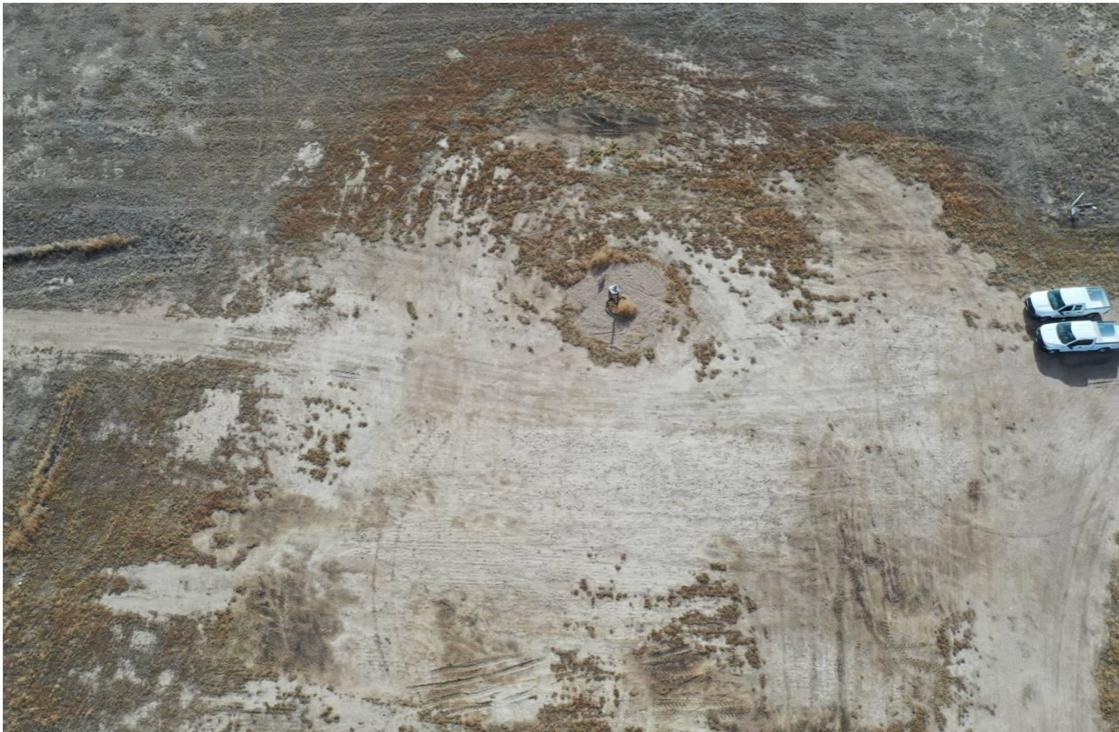
Photo 1. COGCC drone aerial imagery from November 8, 2022. Photo illustrates the Operator has failed to perform subsequent reclamation after Remediation Project #10043 was completed.
