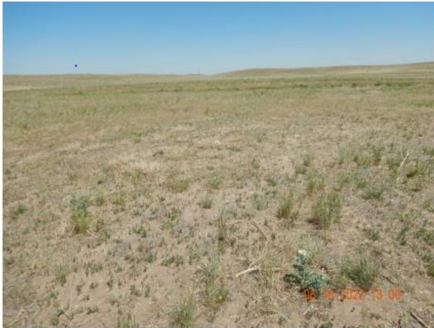
Photo 6. Photo taken from the northern interim reclamation area, facing East. Photo illustrates interim reclamation has been performed; however, an introduced seed mix was used which is not reflective of reference area vegetation per Rule 1003.
