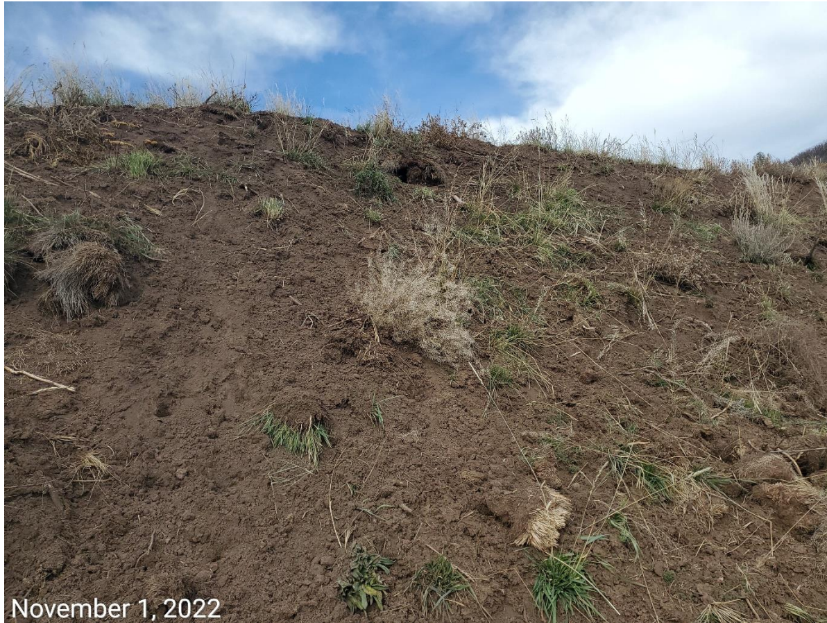
Photo 6: Continued from photo 5. Photo example showing areas of the topsoil stockpile that remains bare, and at risk to wind and water erosion; BMPs to minimize erosion, degradation and sediment transport remain missing or insufficient.
