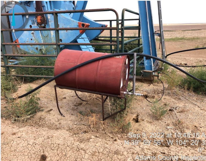
Photo#5 chemical tank outside containment.
