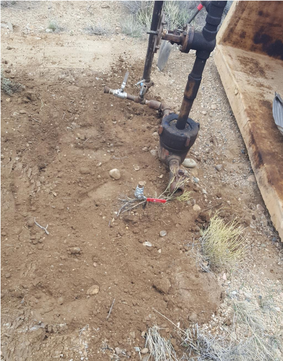
Figure #1 Bradenhead access has been installed.
