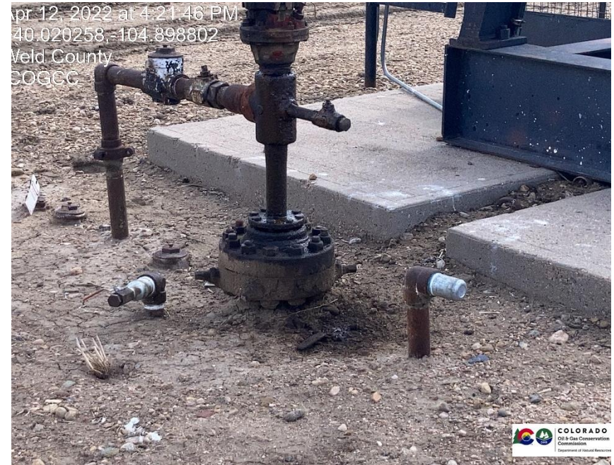
Pic 2 stained soil/mechanical issue with wellhead
