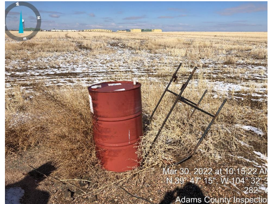
Photo #4 No secondary containment for chemical barrel S/W of well head.
