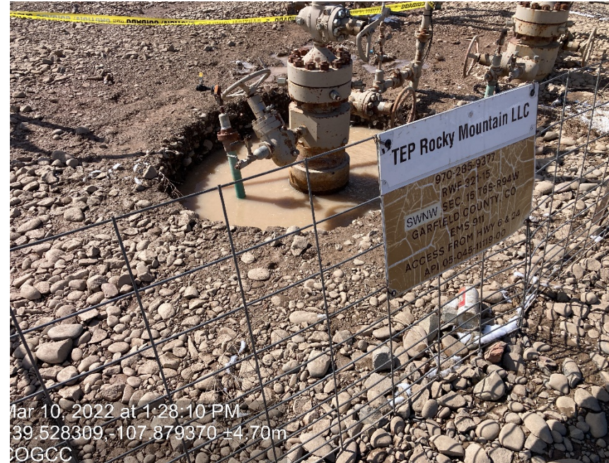
Well head leaking
