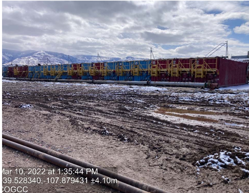
Location/ lack of stabilization-compaction/ open hatches on tanks
