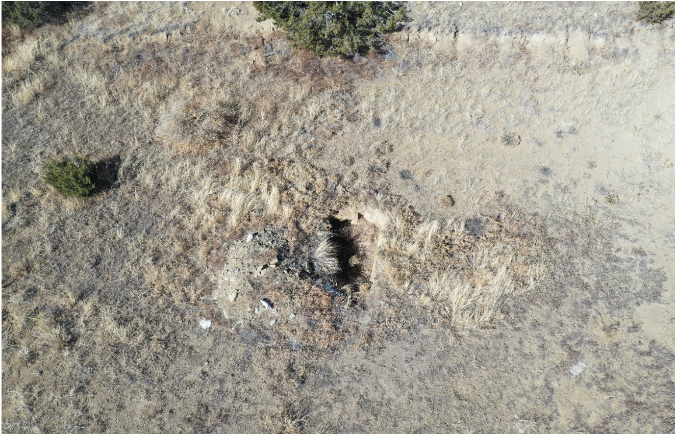
Photo 3. Facing down toward the open hole where the well was cut and capped. The open hole is about 4.5 ft. deep. There is cement debris next to the hole which appears to be from plugging of the well.
