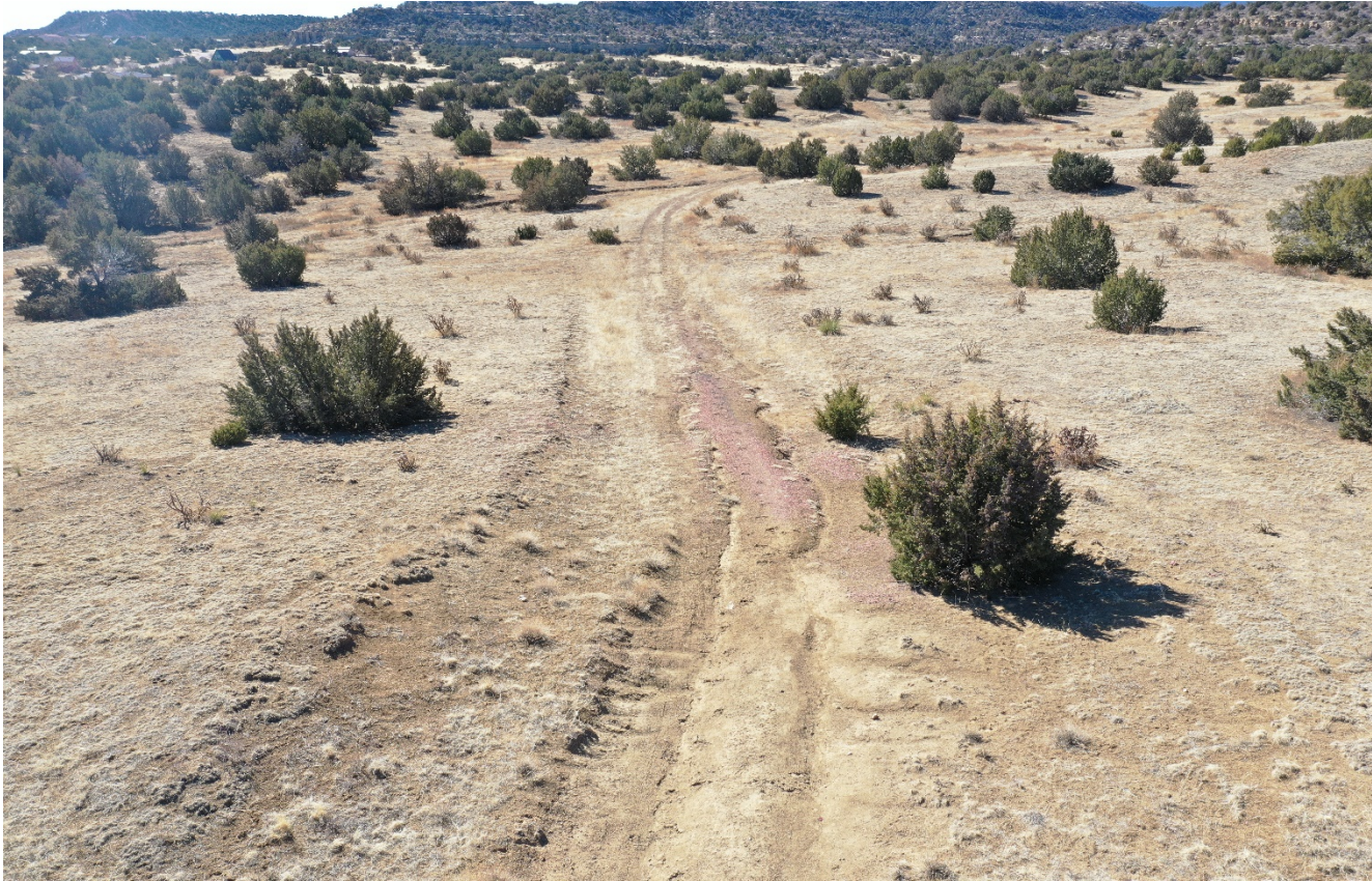
Photo 1. Drone aerial photo facing south along the access road. There is erosion along this area of the road which needs to be repaired and stabilized. Previous corrective action was not performed.
