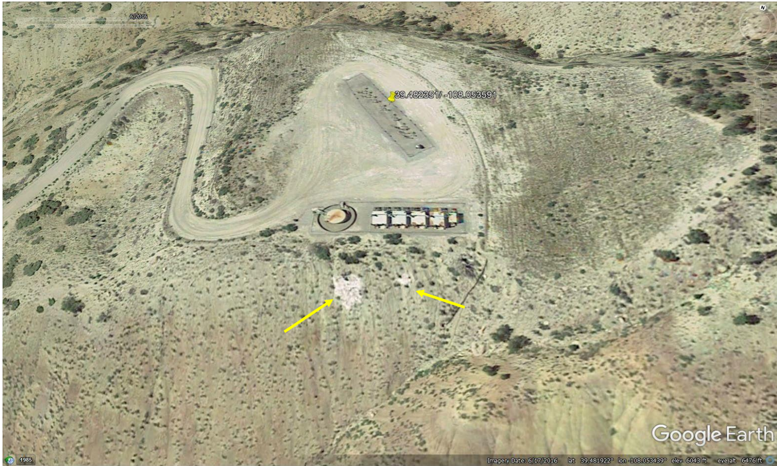
Photo 2: 2016 Google Earth Aerial image. Photo shows potentially impacted soils become evident on the southern slopes of the Location; Sloughing of slopes (see photos 3-6) not evident at this time.
