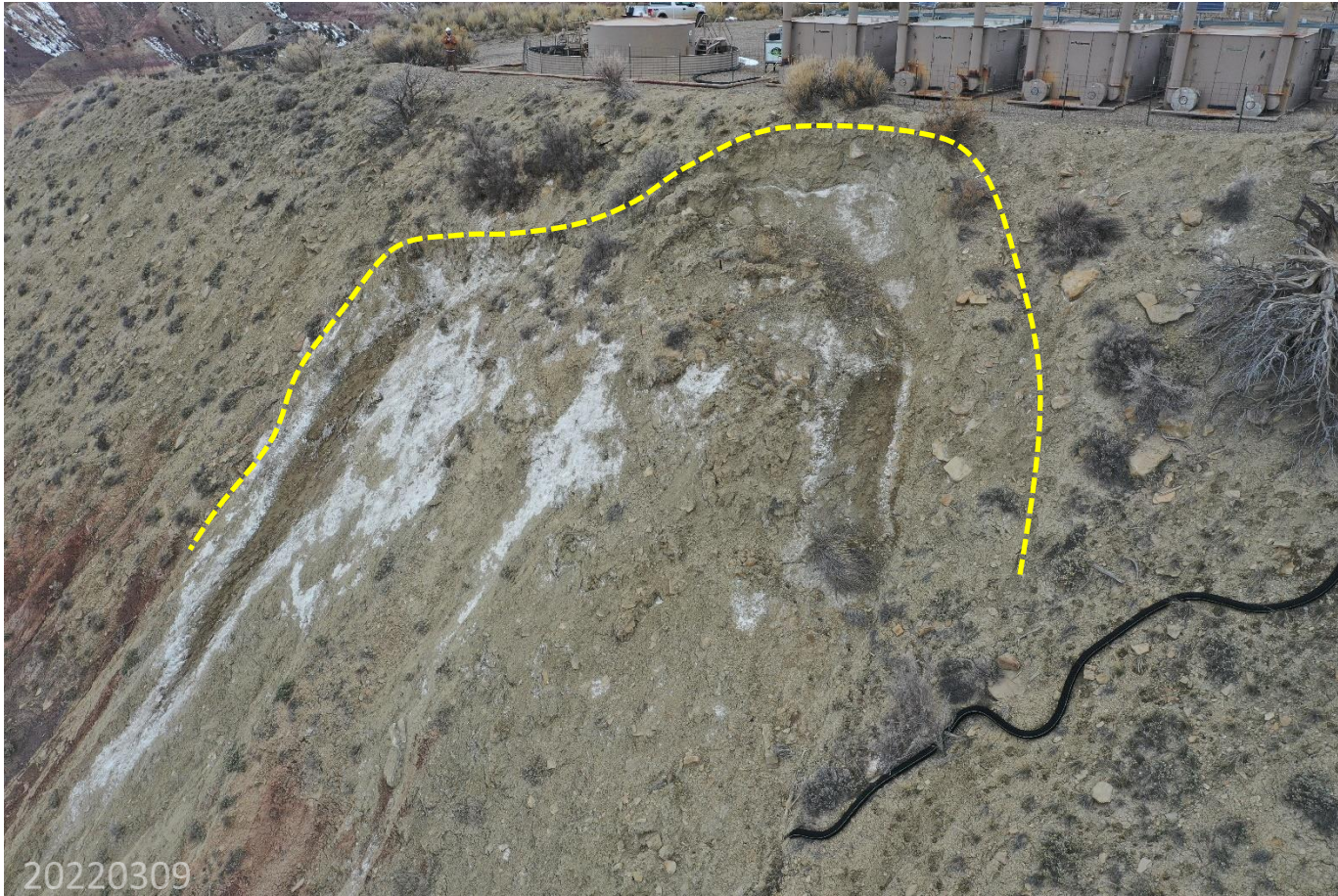
Photo 3: Photos 3-6 taken with use of a sUAS. Photos show large areas of the hillside on the south end of the Location have sloughed off. Photo also shows potential salt impacts; the apparent salt staining appears to be migrating down the slope towards an unnamed drainage. Observed potential salt impact suggests the possibility of a spill originating from below-ground dump-lines or flow-lines at the facility equipment. Additional investigative measures are required by TEP.
