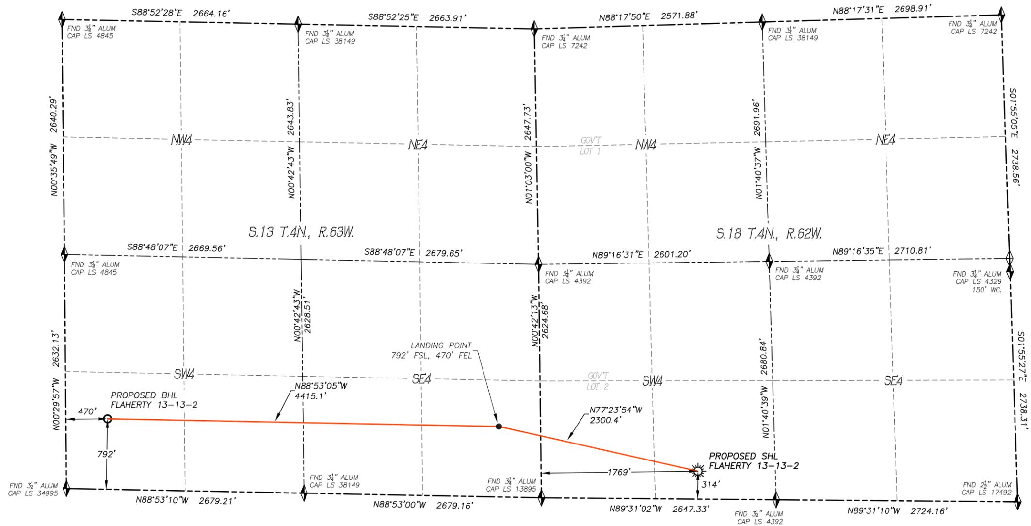
IN ACCORDANCE WITH A REQUEST FROM CONFLUENCE RESOURCES, DALEY LAND SURVEYING, INC. HAS DETERMINED THE SURFACE LOCATION OF THE FLAHERTY 13-13-2 WELL TO BE 314' FSL, 1769' FWL, AS MEASURED AT NINETY (90) DEGREES FROM THE SECTION LINES OF SECTION 18, TOWNSHIP 4 NORTH, RANGE 62 WEST AND THE BOTTOM HOLE LOCATION TO BE 792' FSL, 470' FWL, AS MEASURED AT NINETY (90) DEGREES FROM THE SECTION LINES OF SECTION 13, TOWNSHIP 4 NORTH, RANGE 63 WEST, OF THE 6TH PRINCIPAL MERIDIAN, WELD COUNTY, COLORADO.
