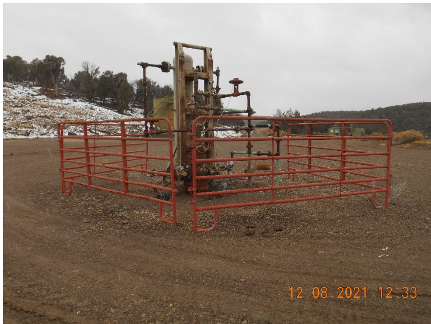
Wellhead with fence with sign.
