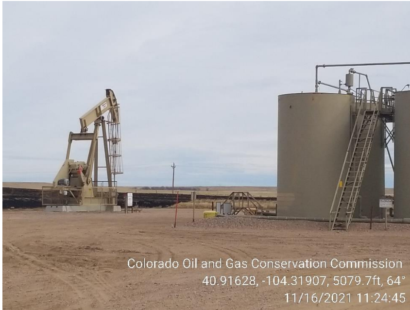
Photo 3 – Tank Battery
