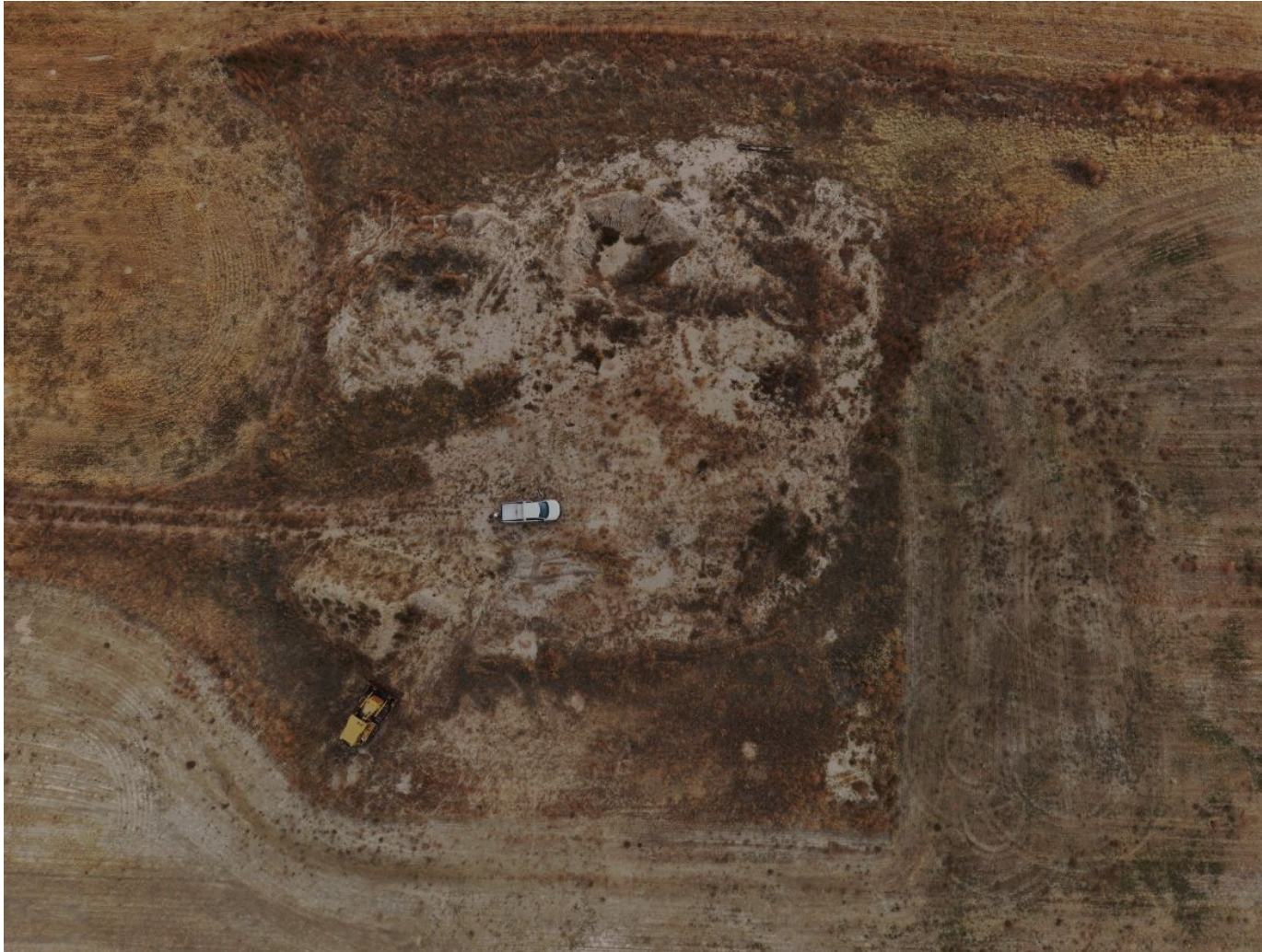
Photo 1. Drone aerial imagery taken of the location. Photo illustrates the Operator has not performed final reclamation, including backfilling a pit.
