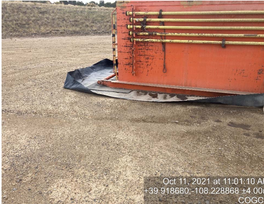
Lack of labeling/failing containment
