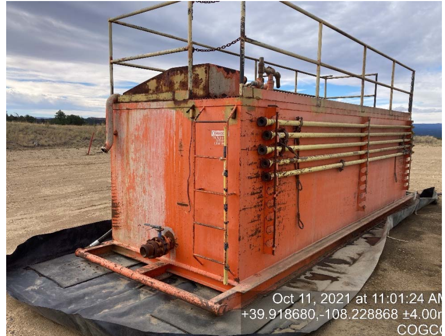
Lack of labeling/failing containment
