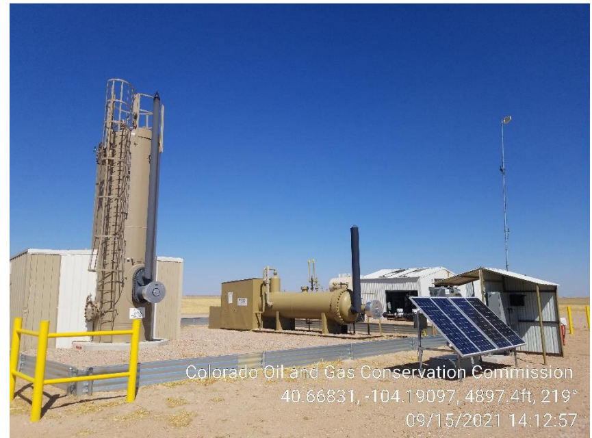
Photo 4 – Separator and Treater
