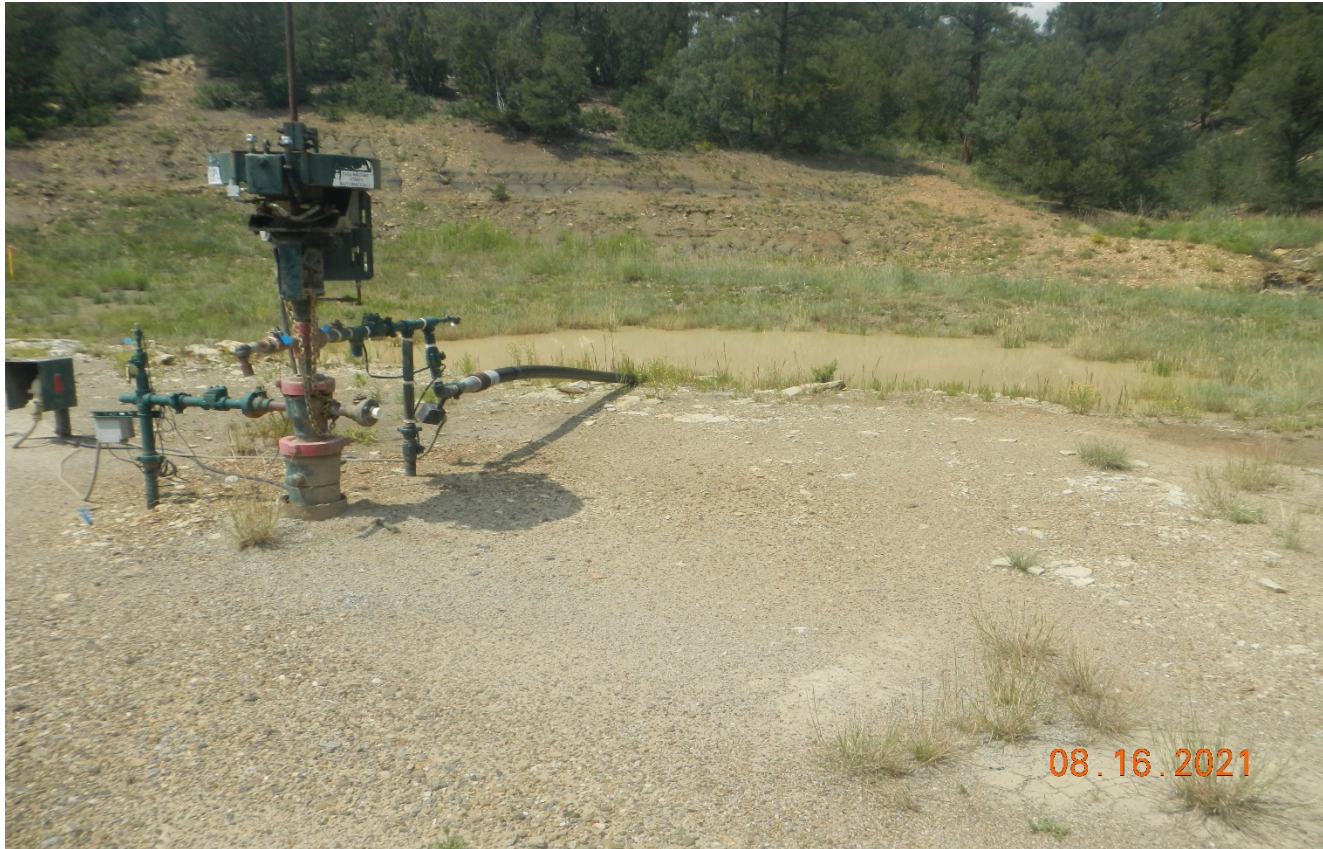
Photo 9. Facing toward the well and pit. Water level is near 2 ft. freeboard and needs to be lowered.
