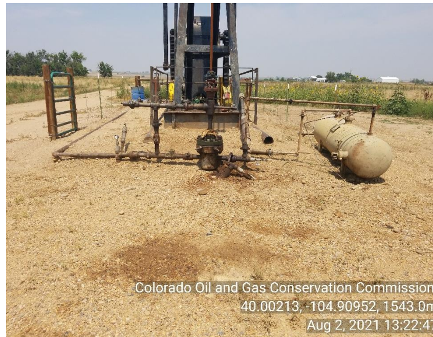
Photo 2 Stained soil in front of and around well head. Well head mechanical issues.
