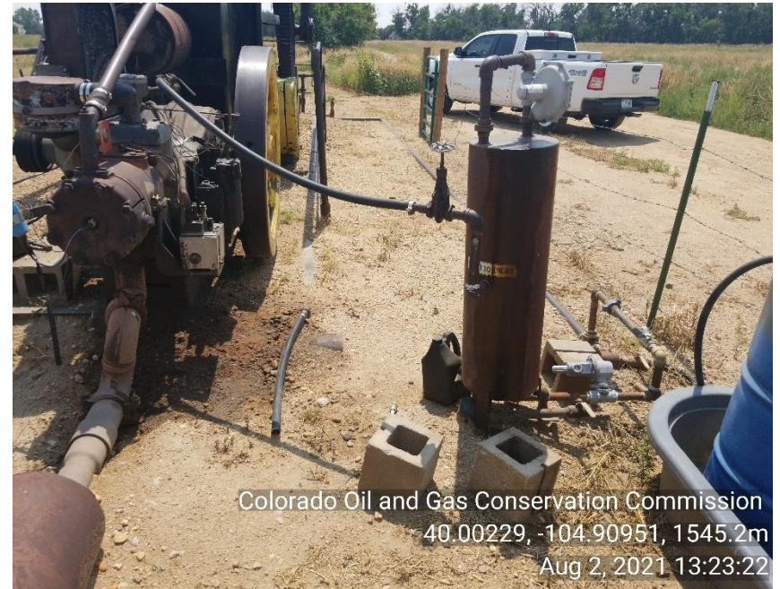
Photo 4 Stained soil and mechanical issues PU motor skid
