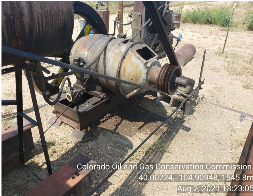
Photo 3 Stained soil and mechanical issues PU motor skid
