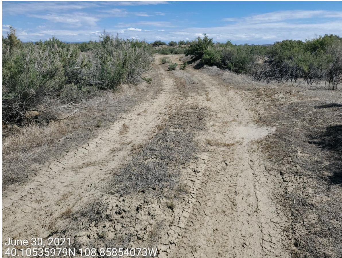
Photo 5: Photo taken from the access road, facing north. Compaction alleviation, recontouring and revegetation activities not performed.
