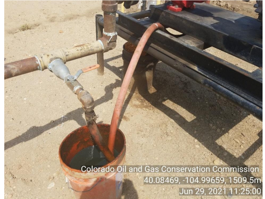
Photo 6 Stained soil and Mechanical issues with recirc pump.
