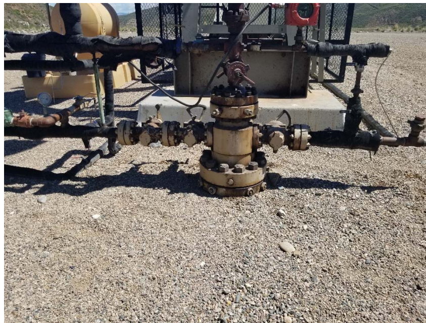
Photo 2. No bradenhead access apparent.
