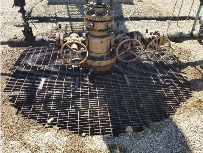
Photo 3. No bradenhead access apparent.
