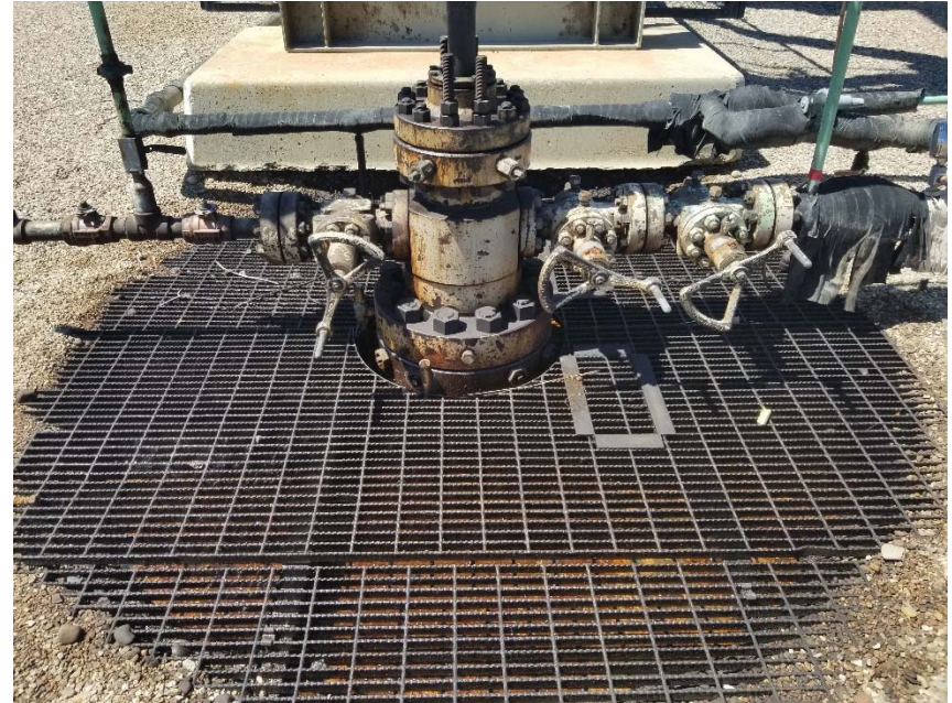
Photo 4. No bradenhead access apparent.
