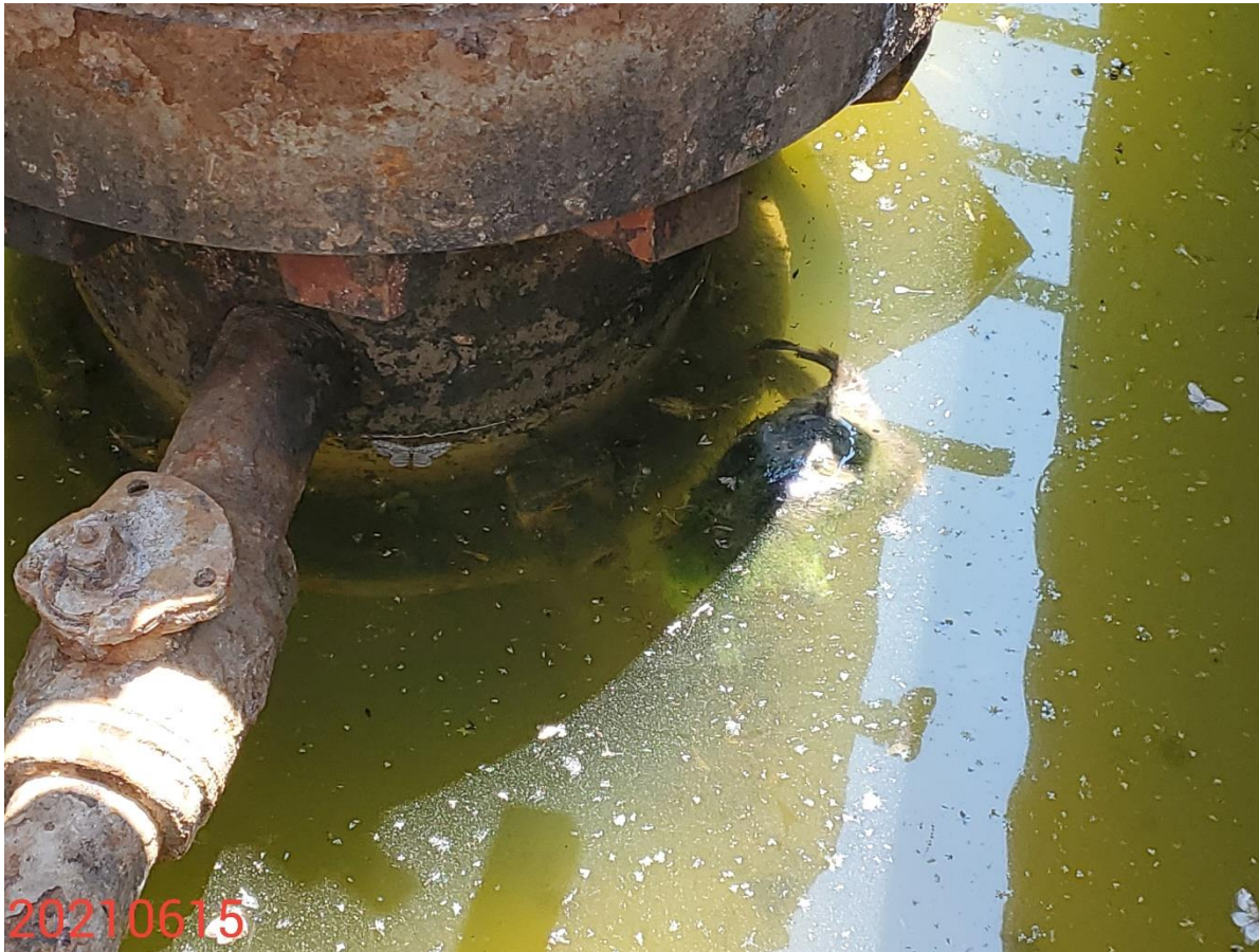
Photo 10: Continued from photo 7. Photo shows wildlife mortality (ground squirrel) within the cellar. Control measures to prevent wildlife access to the cellar, and to protect wildlife resources remain missing or inadequate. Photo also shows fluids/chemicals within cellar have not been removed.
