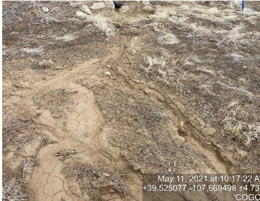
Sediment migration from drain on edge of location
