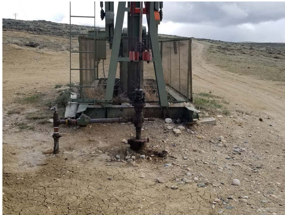
Photo 1. No bradenhead access apparent.
