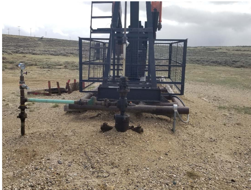
Photo 1. No bradenhead access apparent.
