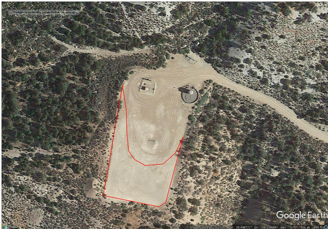
Photo 2: 2019 Google Earth Aerial Imagery. Photo shows pit on the location has been backfilled, however areas of the pad/production area remain unchanged. Photo shows approximate areas on the south end of the Location not needed for production.
