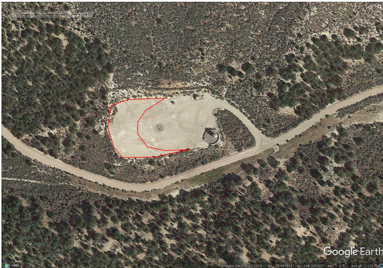
Photo 2: 2019 Google Earth Aerial Imagery. Inspection dated 11/12/2013 required Operator to conduct interim reclamation. Imagery shows pit on the location has been backfilled, however areas of the pad/production area remain unchanged. Photo shows approximate areas on the west end of the Location not needed for production.
