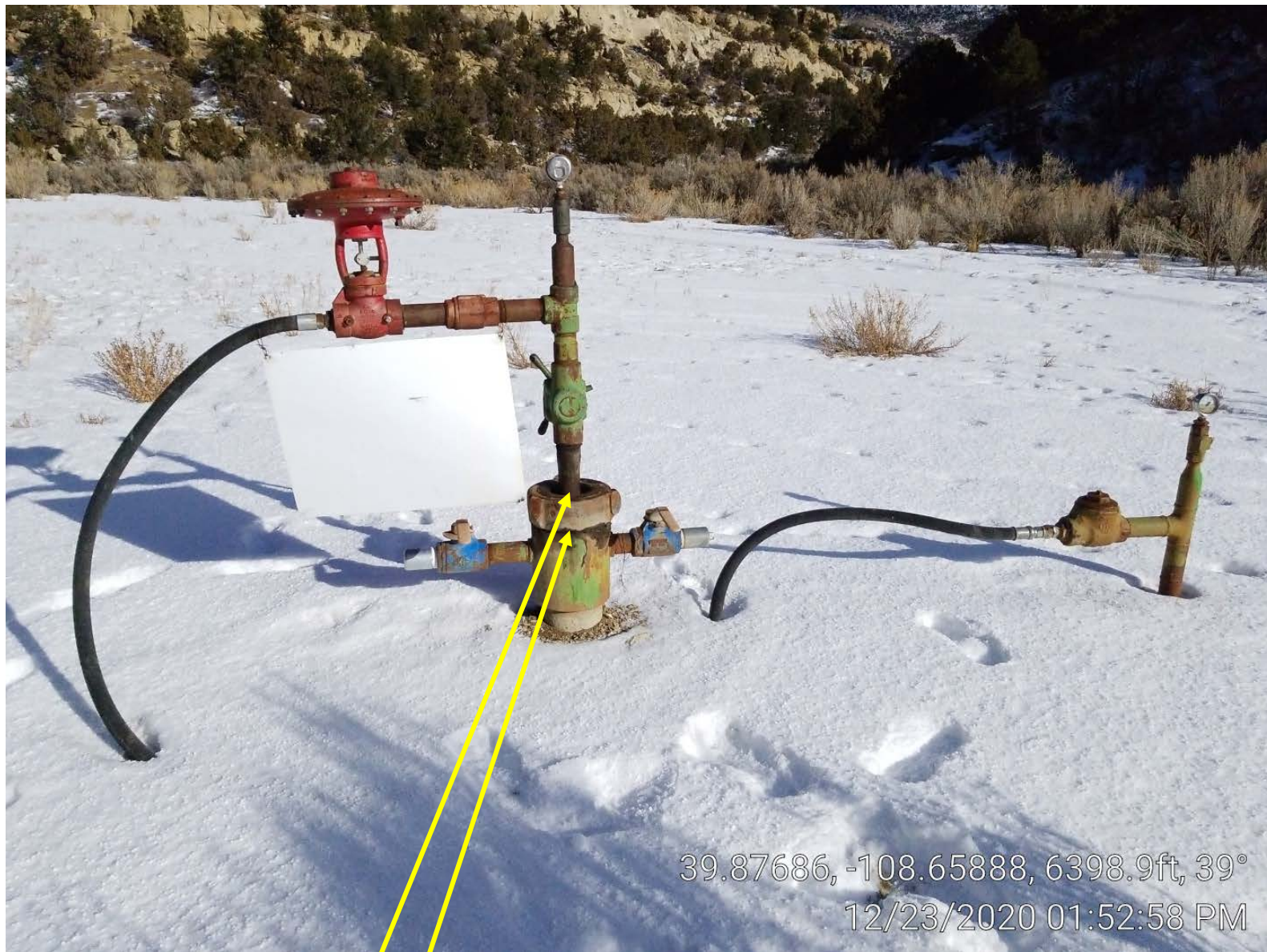
Photo 2. Well gas leaks.
