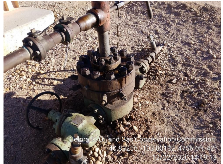
Photo 8 – Stained Soil at Wellhead
