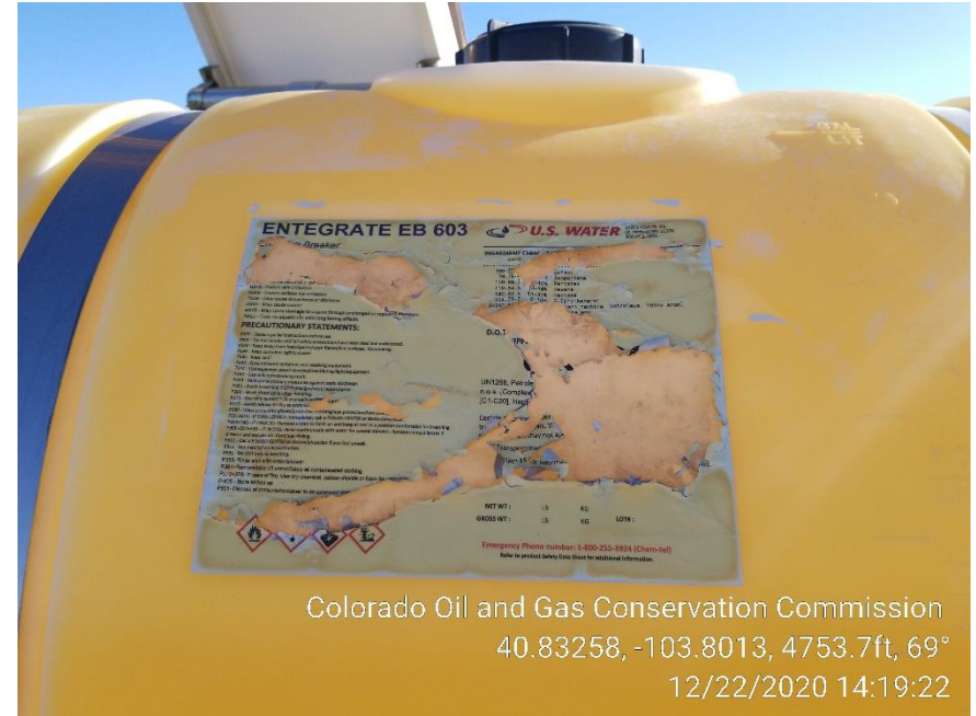
Photo 6 – Label on Chemical Container has faded
