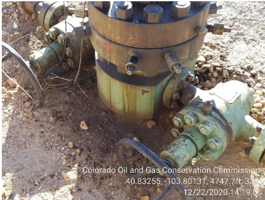
Photo 7 – Stained Soil at Wellhead
